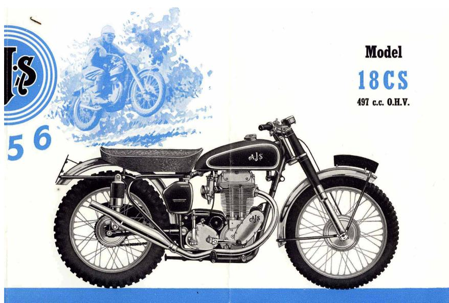
Special attention has been paid to the question of suspension and steering in order that full advantage may be taken of the high maximum power and colossal acceleration provided by the new short stroke racing-type engine.
