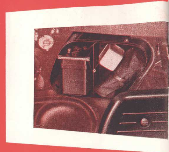
New tool box and battery carrier fitted to all single cylinder models
