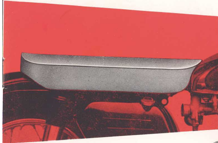
Re-designed dual seat fitted to Models 50, ES2 and 19S
