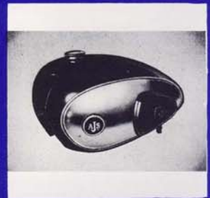
Petrol tanks featuring chromium plated side panels enhance the appearance of the twin models.
