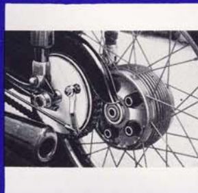
New quickly detachable rear wheel incorporating cushioned rubber drive.
