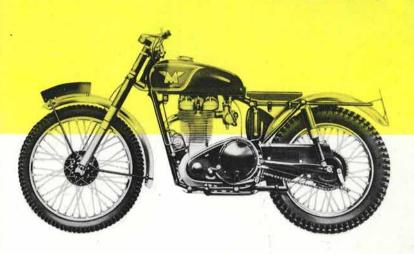
The 350 c.c. Trials MAESTRO. One of the few machines initially designed as a trials model—and now fitted with the works type short-stroke engine.
