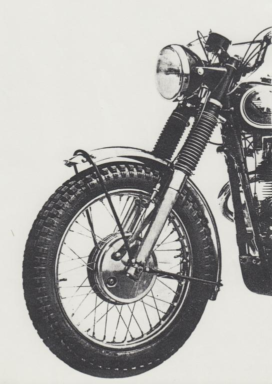
for scrambling: give extra long movement and precise progressive two-way damping: multi-rate springs: large diameter heat-treated tubular steel stanchions: alloy sliders: rubber gaiters: forged steel handlebar lug and fork crown: crown pinch bolts act as steering lock stops.
