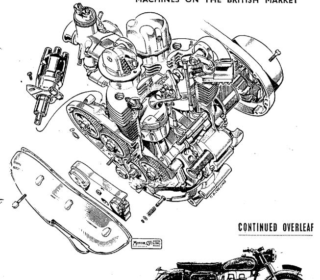
Latest edition of the A.M.C. parallel twin is the 650 c.c. version shown above with its normal touring crankshaft generator and coil ignition distributor. For scramblers, such as the A.J.S. Model 31CS seen on the right, magneto ignition is specified and a quickly detachable dynamo is carried athwart the front of the engine. A.M.C.s are alone in employing a centre bearing on a big-capacity o.h.v. power unit of this type.
