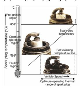
The firing end appearance also depends on the spark plug tip temperature. There are three basic diagnostic criteria for spark plugs: good, fouled and overheated. The borderline between the fouling and optimum operating regions (500&def;C) is called the spark plug self-cleaning
