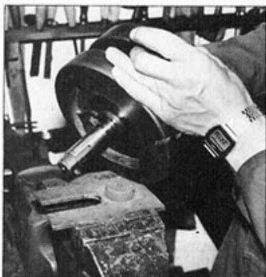
Time spent making up a jig to hold the crank is time wisely invested. A slot in this 1/4-in steel plate accepts the mainshaft; a stub locates the flywheel cut out.
