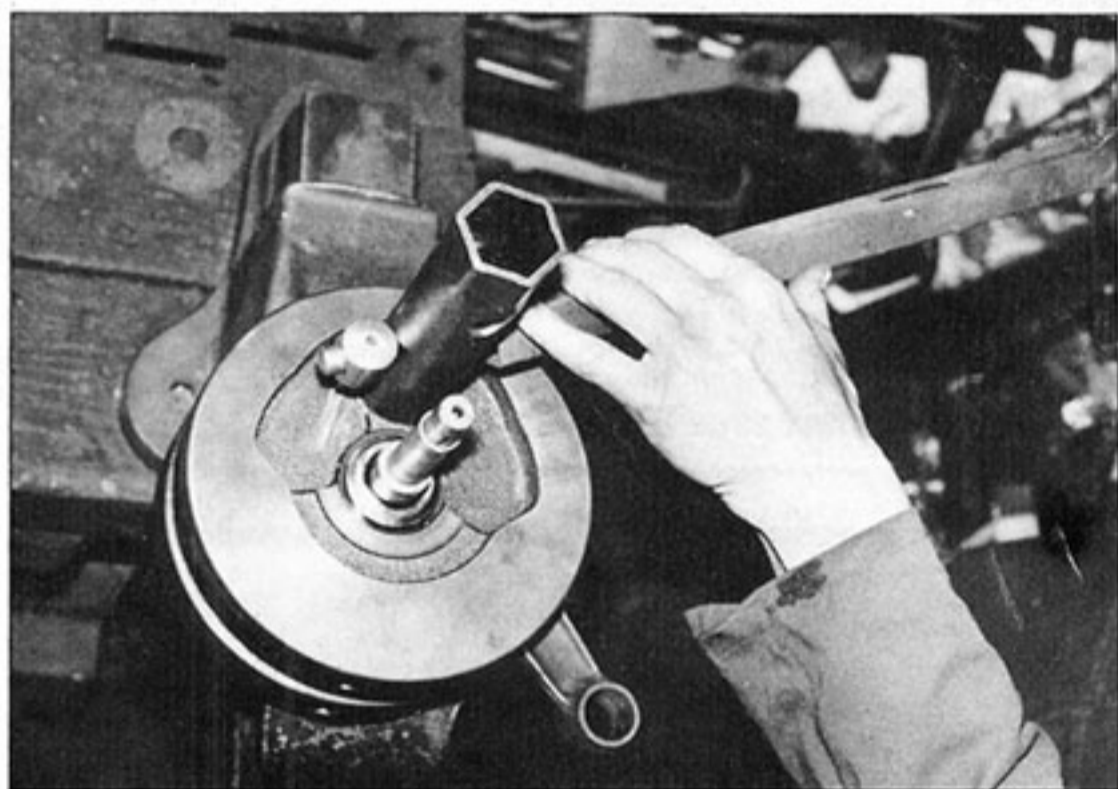
Above: Crankpin nuts are tight, so use a jumbo size box spanner or a tight fitting socket.
