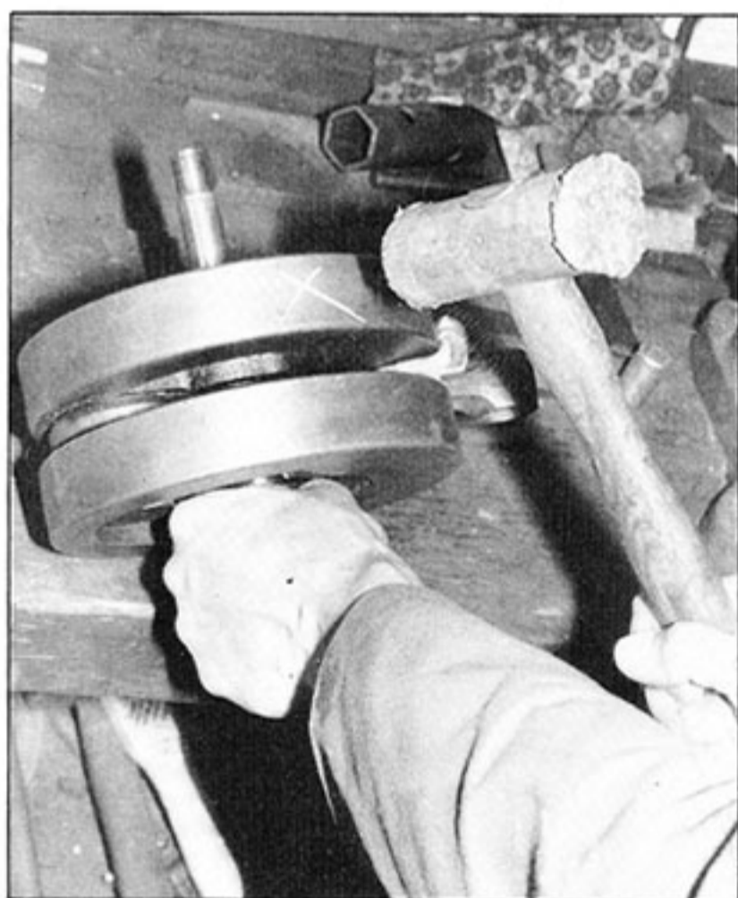
Rest the back of the opposite wheel on the bench. X marks the spot to hit before you put it back in the jig. Tighten and lock the final nut only when the result surpasses perfection.
