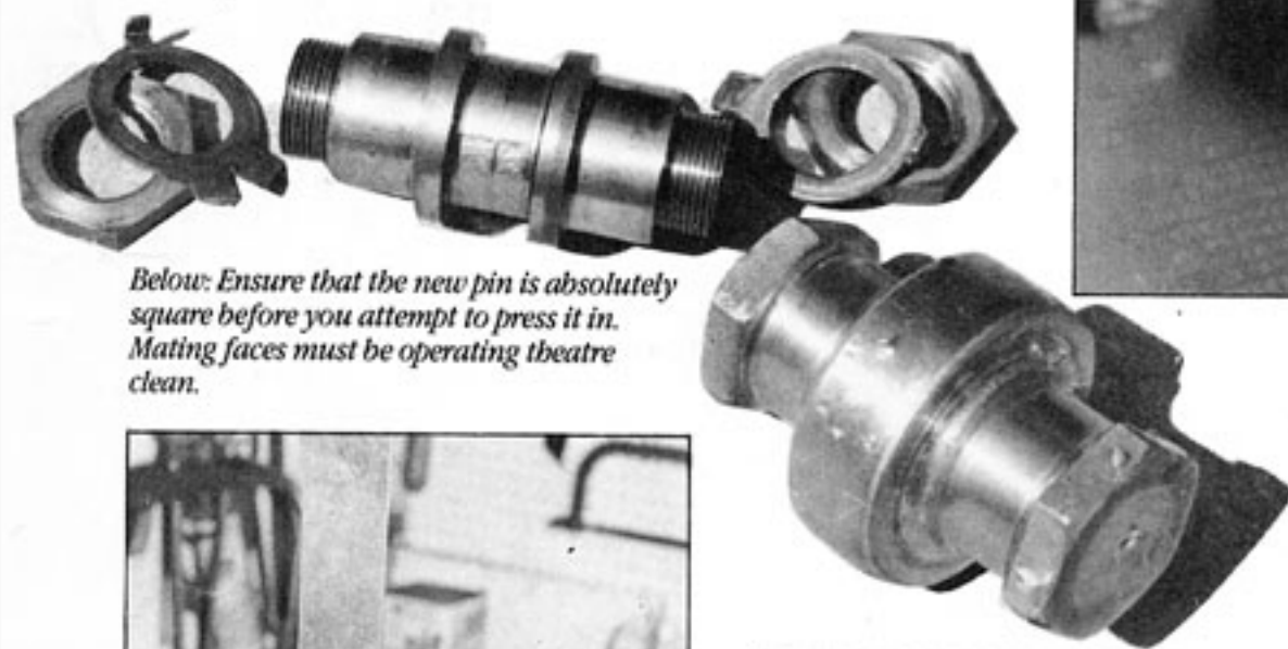
Right: Out with the old; in with the new. Big-end track renewal is a two-in-one operation.
