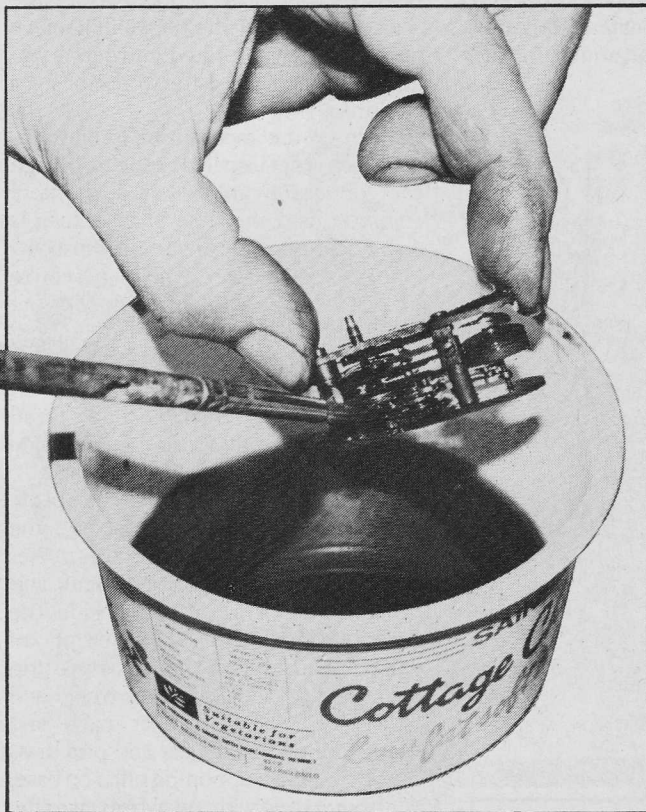
Worm on drive shaft turns gear A, and eccentric drive to the pawl B, which turns the recording drum ratchet.
