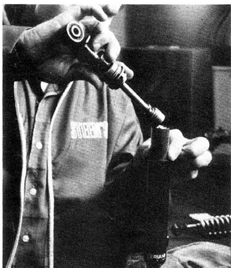
Push the damper rod in very slowly, all the way to the bottom of the cylinder. Let the overflow run inside the housing.
