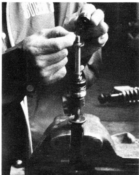
This spring washer goes on next and then the 12mm nut. Tight.
