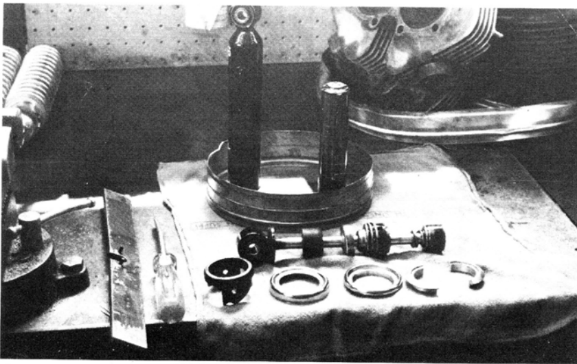
The damper rod will pull out easily — if it isn't bent. Get it out and then remove the cylinder, drain the old fluid and clean the parts.
