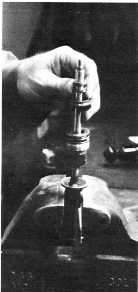
Position what you've got so far and then slip on the flow block and spring.
