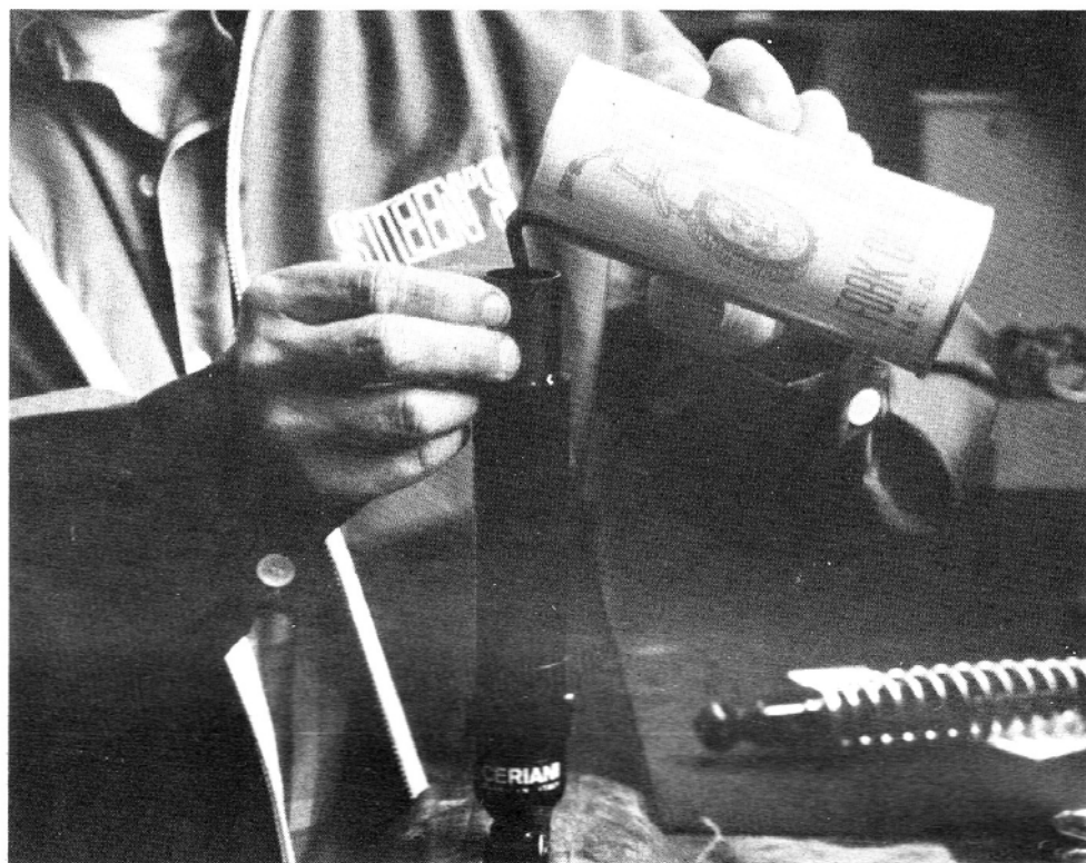
Fill the internal cylinder with about two ounces of hydraulic fluid.
