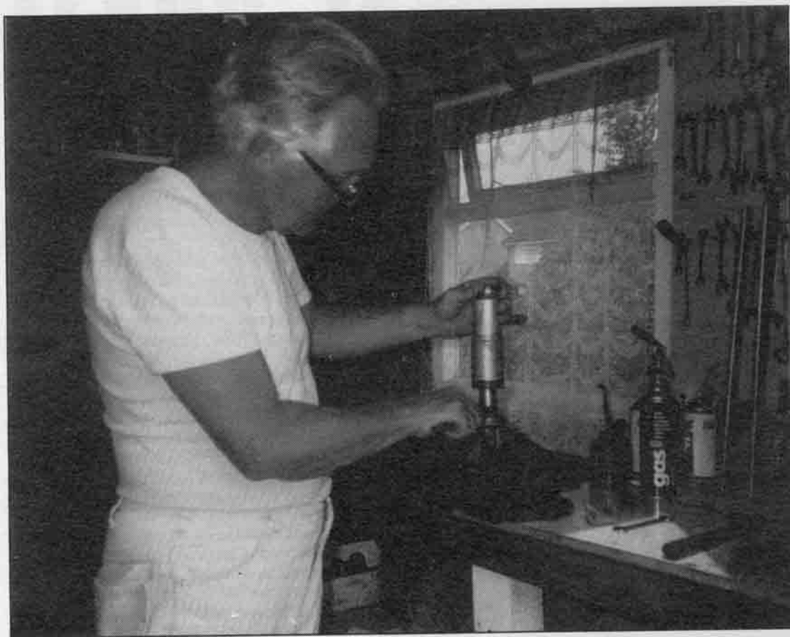
Fitting inner tube to upper pivot, gripping part of tube normally covered by rubber buffer. "Parallel bars" tool on bench, extreme right.
