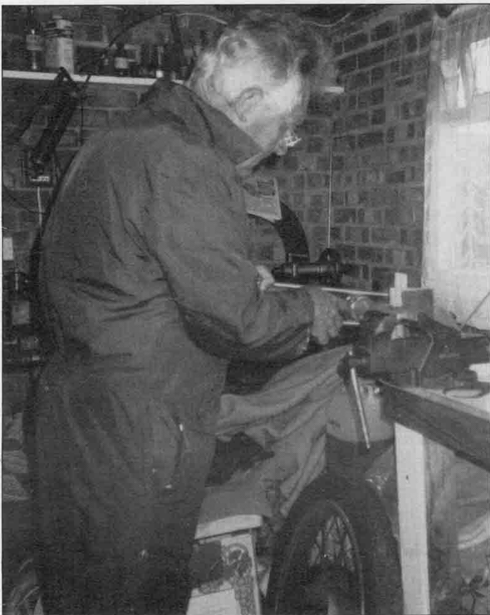
Using the "parallel bars" spring compressor.
