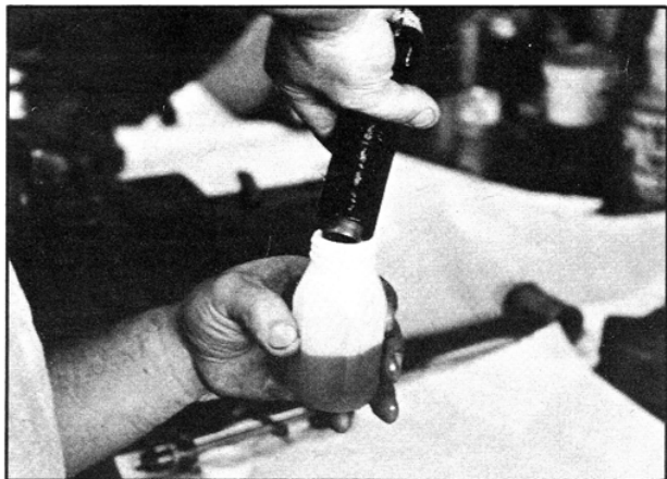
Dump the old oil into a measuring device. That way you'll know how much was in there.
