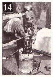
its ability to retain oil and the MoT test is getting more stringent in this regard. If there are signs of leakage around the unit the bike will be failed. At £20.54 (inc VAT) for a pair of new inner tubes, not to replace them is false economy. Then there's 10 percent off for members of the owners club.
