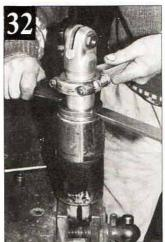
Before removing bottom pivot turn unit upside down and put top pivot in rod is to grip the outer tube with a Ubolt and bar being careful to place leather the vice, (pic 29) the reason being to prevent oil from gushing over the old carpet padding between bolt, bar and the outer tube body. This second method isn't as slippers. • Remove bottom pivot (pic 30), satisfactory because the full circumference of the tube is not gripped,
