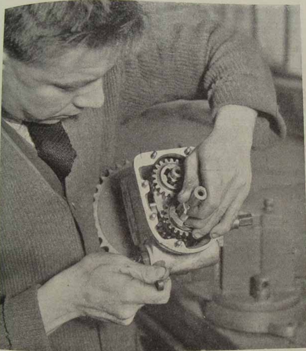
Fig. 6.—HOW THE LAY SHAFT AND BOTH SLIDING PINIONS ARE FITTED INTO POSITION TOGETHER. NOTE HOW THE PEGS ON THE SLIDING GEARPLATE ARE BEING ENGAGED WITH THE SLOTS IN THE OPERATING FORK.
