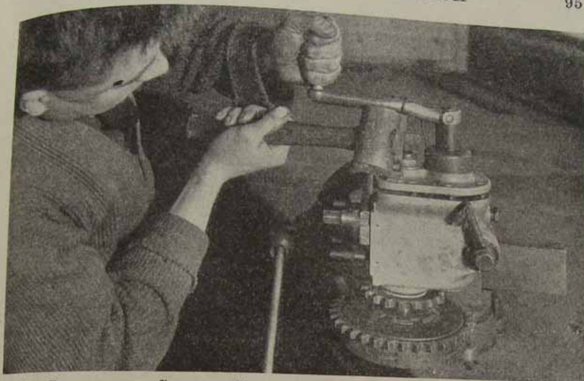
Fig. 3.—REMOVING THE GEARBOX COVER, AND PARTING THE OILPROOF JOINT WASHER.
