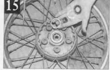
the brake drum face down on the bench. Remove the circlip which retains the bearing with the aid of a screwdriver (pic six). Then remove retaining washer.
