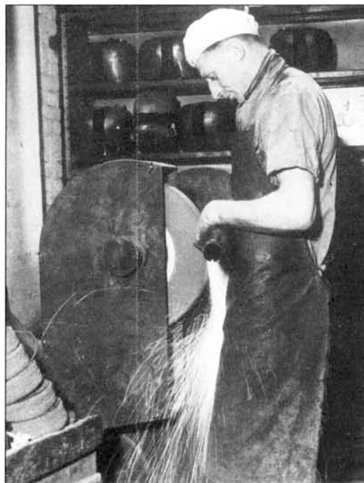
An exhaust silencer is put through the rough grinding process at Plumstead in 1948
