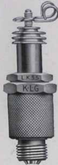
"K.L.G." Type L.K.S.5 PLUG 14 m/m. diameter thread, short (10 m/m.) reach, two-piece detachable model for sports cars and sports motor cycle engines where "small" plugs are required. Fitted with radiator cooling fins. No. SP533/500 ... each 7/6 SP533/406 (4 doz. rate)
