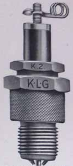
"K.L.G." Type K.2. PLUG Metric thread, \frac{3}{4} in. reach, two-piece detachable model. This plug is the long reach equivalent of the K.1. Fitted with one or three earth points as preferred. No. SP526/400 ... .. each 6/- SP526/307 (4 doz. rate)
