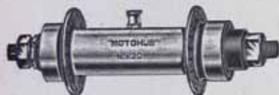
MOTOR-CYCLE FRONT HUB Width over flanges, 3". Width over cones, 4". Spindle diameter, 1/2". Drilled 36 holes. No. HU30/500 ... .. each 6/8
