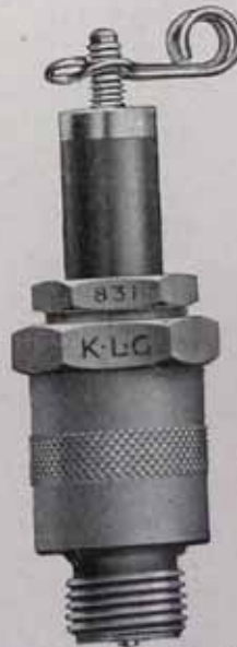
"K.L.G." Type 831 PLUG 14 m/m. diameter thread, short (10 m/m.) reach, two-piece detachable model, two earth points. This model was designed for all 1935 Standards with the exception of the "Sixteen" and "Twenty." No. SP541/400 ... each 6/- SP541/307 (4 doz. rate)
