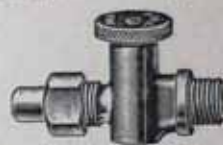
"EVERTITE" PETROL TAP Patent cork-seated and adjustable. To open, pull knob, to close, push knob. To adjust, remove hexagon lock nut and with a small screwdriver turn the adjusting spindle for half or full turn, replace lock nut and tighten up securely. No. Nickel-plated. TA220/103 \frac{1}{4} " gas x \frac{1}{4} " gas each 1/10 TA221/103 \frac{1}{4} " gas x \frac{3}{8} " gas .. 1/10
