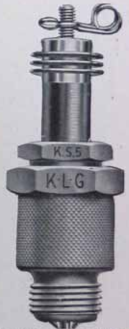
"K.L.G." Type K.S.5. PLUG Metric thread, \frac{1}{2} in. reach, two-piece detachable model fitted with radiator cooling fins intended for high efficiency and sports car and motor-cycle engines. No. SP529/500 ... .. each 7/6 SP529/406 (4 doz. rate)
