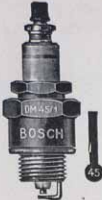
BOSCH DM45/1 PLUG For low compression engines. Extended insulation gives longer reach. Thread length, 12 m/m. No. Barrel length 12 m/m. SP280/206 ... each 4/6
