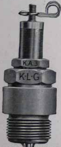
"K.L.G." Type K.A.3 PLUG American thread, \frac{1}{2} in. reach, two-piece detachable plug specifically designed for engines with A.L.A.M. threaded plug holes. Fitted with one or three earth points. No. SP527/400 ... .. each 6/- SP527/307 (4 doz. rate)
